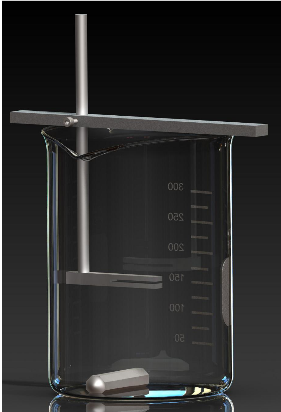
Figure 8. Illustration showing one of the Teflon substrate holders utilized in hydrothermal growth.
